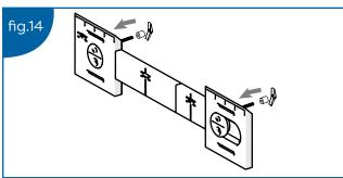
iii) Insert the threaded bolt through the Hang 'N' Lock cams and reattach the plugs and spring. (See Fig. 14)
