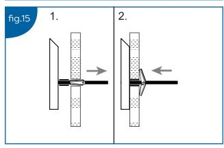
iv) Push the spring loaded wall braces on the toggle bolts through the drilled holes and loosely secure the Hang 'N' Lock bracket to the wall. (See Fig. 15)
