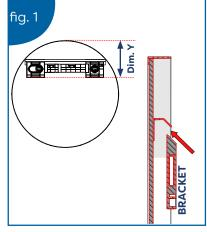
2 Carefully hold your mirror in the desired location and using a pencil, draw a reference line along the top edge of the mirror. Use the bracket distance vou measured earlier to create a reference line for the bottom of your Hang 'N' Lock bracket. (See Fig. 2)
