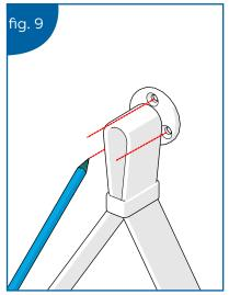
Drill the marked holes to a depth of 45mm with a 6mm drill bit. Insert wall plugs level with the surface of the wall. For tiled surfaces, insert the wall plugs below the surface of the tiles to avoid cracking. (See Fig. 10)
