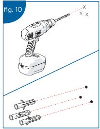
Insert screws through the hook bracket and fasten in place. Once secure, place the cover over the bracket and screw on the hook.
