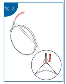
Place the hook bracket behind the loop of the strap and mark hole centres using a pencil.
